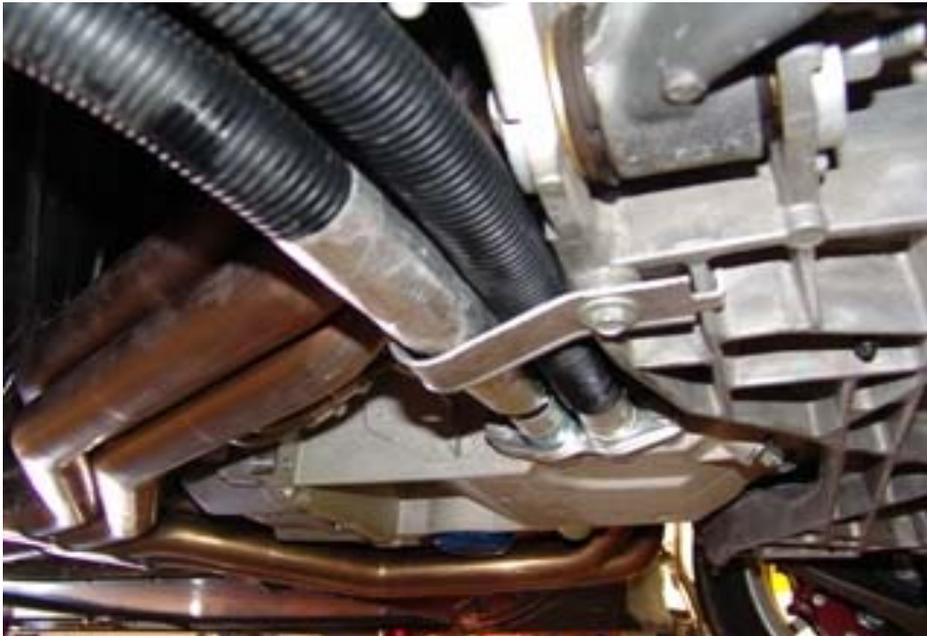
**Figure 1: Oil line clearance after bracket has been bent.**
