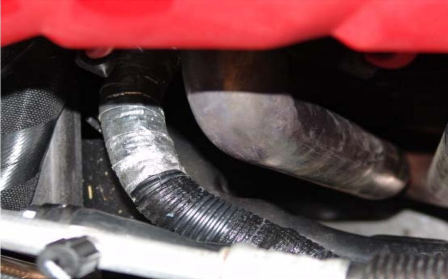
**Figure 2: Passenger side wiring harness after being relocated**
