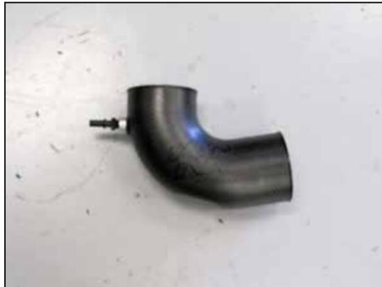
14. Install the provided NPT quick disconnect fitting into the K&N intake tube as shown.
