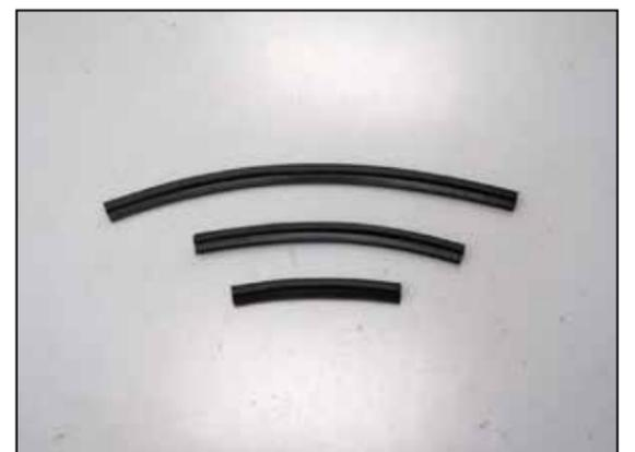
6. Cut the provided edge trim into three sections of 24", 15" and 9" as shown.
