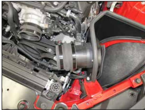
13. Install the provided hump coupler hose (084101) onto the mass air sensor housing and secure with the provided hose clamp.
